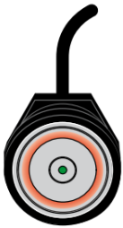
Reader LED turns amber (programming mode)
