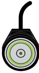
Reader LED turns green (enrolled key)
